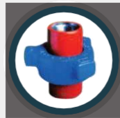
Fig. 2202 Green Nut Green Subs Especially for sour gas service; with heat-treated components, fluoroelastomer seal rings. For service to 15,000 psi NSCWP*.
