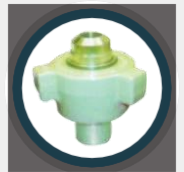
Fig. 2202 Green Nut Green Subs Especially for sour gas service; with heat-treated components, fluoroelastomer seal rings. For service to 15,000 psi NSCWP*.
