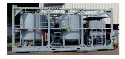
Construction Two number of tanks – Skid or Trailer mounted
